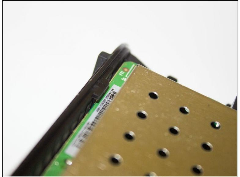
**⚠** Don't pull too fast! Some clips get in the way of the board, and you have to clear them by bending the outer frame slightly outwards.
