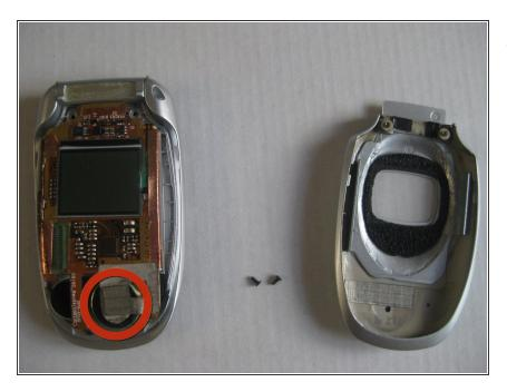
The speaker is covered with silver tape on the bottom of the logic board.
