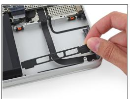
• Tilt the outer hard drive bracket up toward the logic board and remove it from the rear case.
