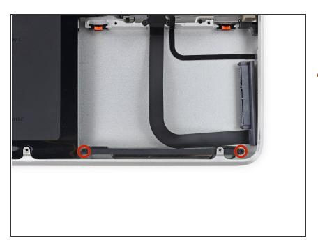
Remove the two 5 mm Phillips #00 screws securing the hard drive bracket to the upper case.
