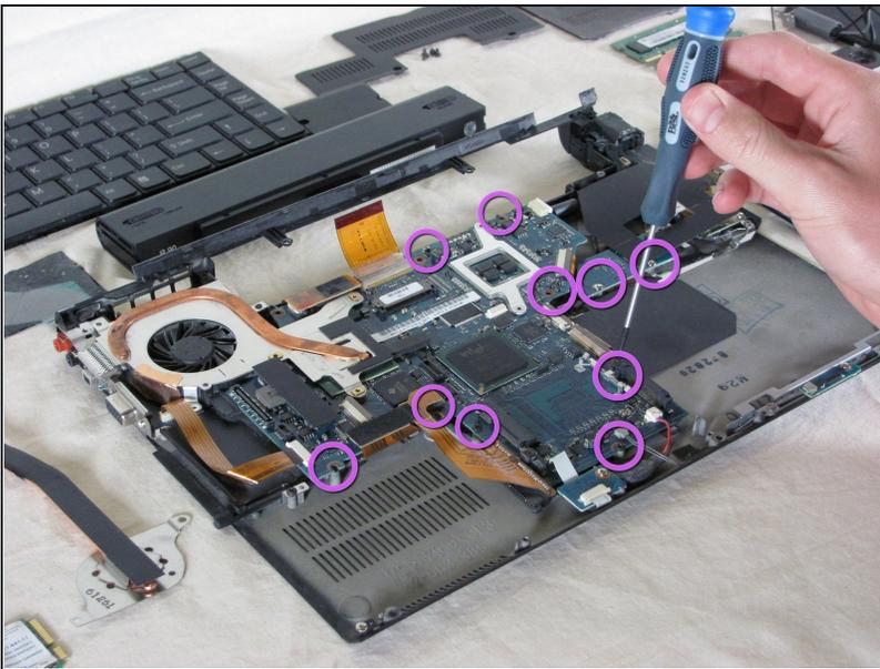
**⚠ Caution:** Ground yourself before removing the logic board. Static electricity can damage the logic board.
