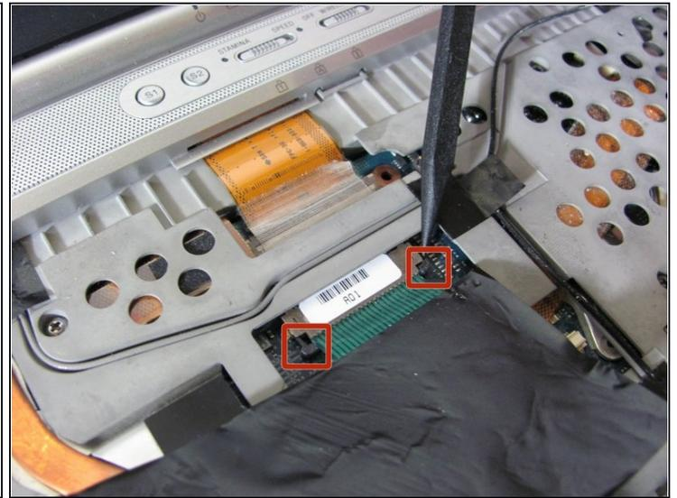
**⚠** The keyboard is still attached by ribbon cable, don't try to remove the keyboard entirely yet.
