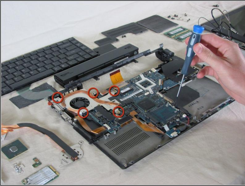
**⚠ Caution:** When removing the fan, be careful to not tear the attached ribbon cable.
