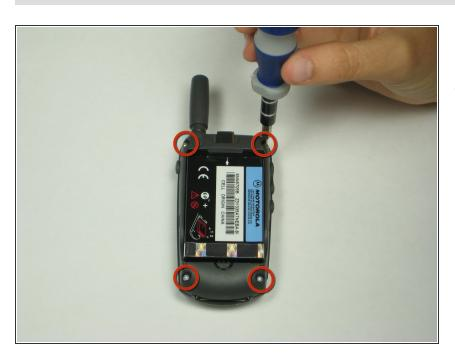
Using a T6 Torx screwdriver, remove the four screws from the back of the phone.
