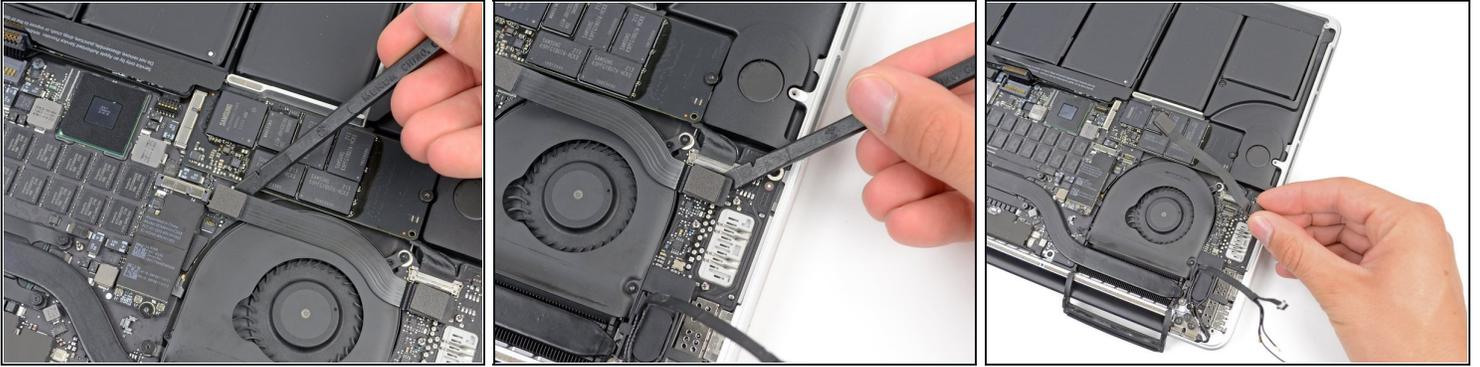
ⓘ If your I/O Board cable's connectors have [notches in the padding](#), you will need to **release a locking lever underneath the notch** in order to remove the cable. If this is the case, **don't pry up on the connector until the levers are unlatched**.
