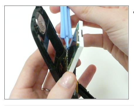
Use the opening device to remove the ribbon wire where it connects to the screen.
