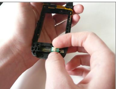
Remove the black sim card reader and green vibrator before continuing to ensure they do not fall out.
