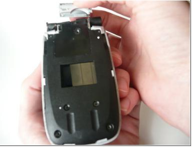
Use the opening tool to pry up the edge of the remaining silver hinge cover. Once it is loose, pull it
