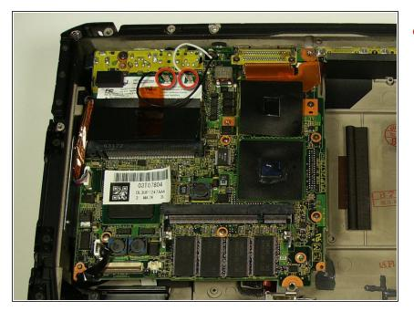
Remove the black and white wires attached to the wireless card by simply pulling up.
