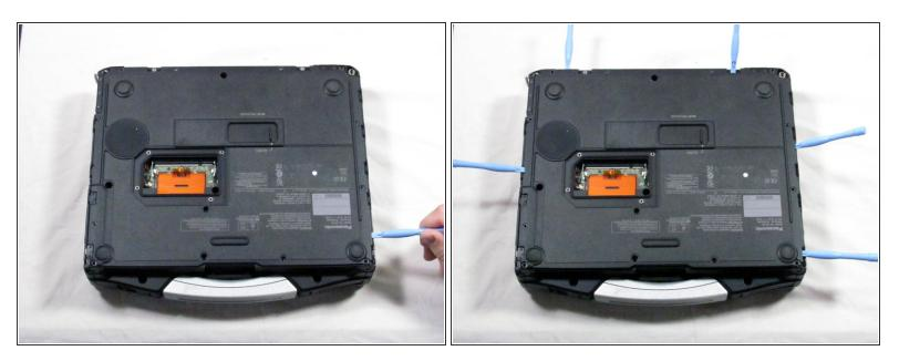
Use a plastic opening tool to release, but NOT remove, the back cover because it is sealed with adhesive.
