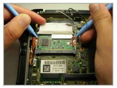
Using a pair of plastic opening tools, push the two metal tabs away from the card.
