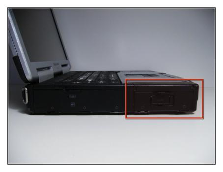
• Locate the bay door for the battery on the left side of the laptop.
