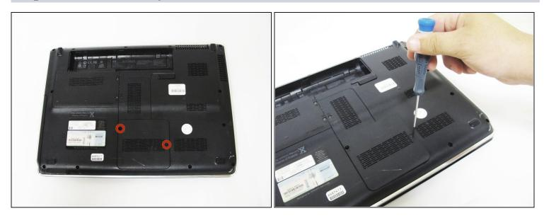
• Remove these two 4mm Phillips screws on the back panel using a Phillips #00 screwdriver and remove the cover to reveal the CMOS battery
