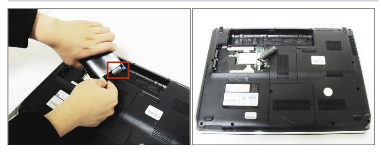
• Gently lift the ribbon cable away from the hard drive enclosure to free the drive.
