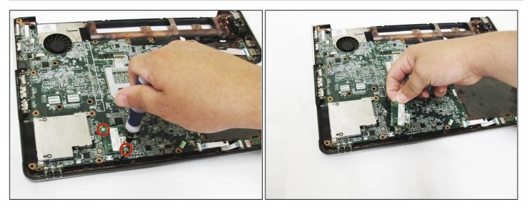
• Using the Phillips #00 screwdriver, unscrew the spring-release fasteners on the modem card and remove it from the board.
