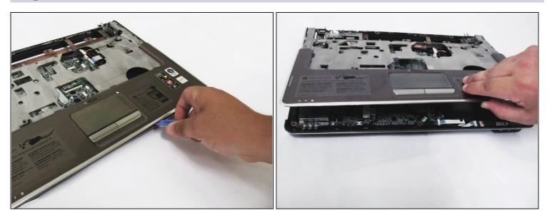
• Using a plastic opening tool, carefully pry off the top plastic cover by lifting it up at the seam at various points around the edge, then remove it completely.
