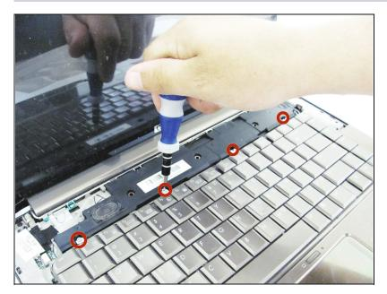
Use a <u>2.5mm flathead</u> screwdriver to remove the four 3mm screws on top of the keyboard.
