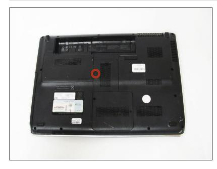
Remove the one 4mm Phillips screw from the RAM cover using a Phillips #00 screwdriver.
