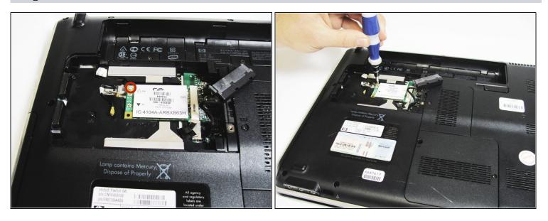
• Locate the 2.5mm Phillips screw on the corner of the WLAN card and remove it using a Phillips #000 screwdriver.
