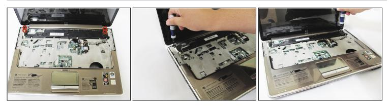
• Locate four 3mm screws in the upper corners of the keyboard tray and remove them using a #00 Phillips screwdriver.
