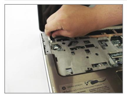
Locate the large display ribbon connector near the upper left corner of the keyboard tray and remove the ribbon by pulling straight out on the connector.
