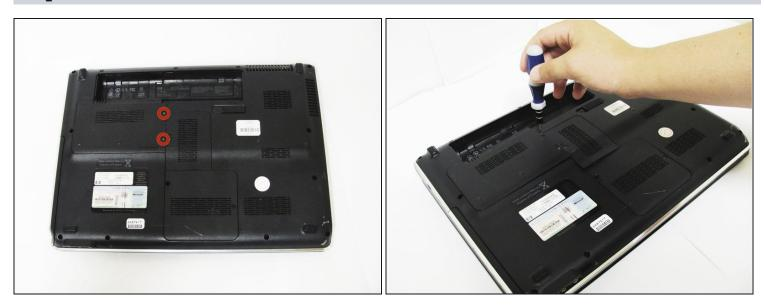
• Remove the two 5mm Phillips screws on the hard drive cover using a Phillips #00 screwdriver.
