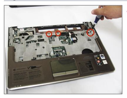
• Remove the three 3mm Phillips head screws on the top of the frame using the Phillips #00 screwdriver.
