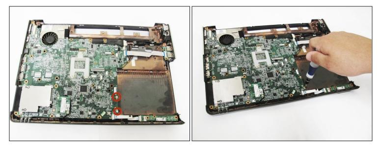
• Remove the two 2mm screws on the bottom right of the motherboard using the Phillips #00 screwdriver.
