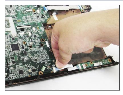
• Remove the ribbon on the bottom left of the board.
