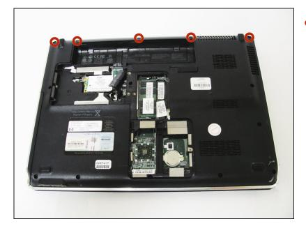
Remove the five remaining 2mm screws using a Phillips #00 screwdriver.
