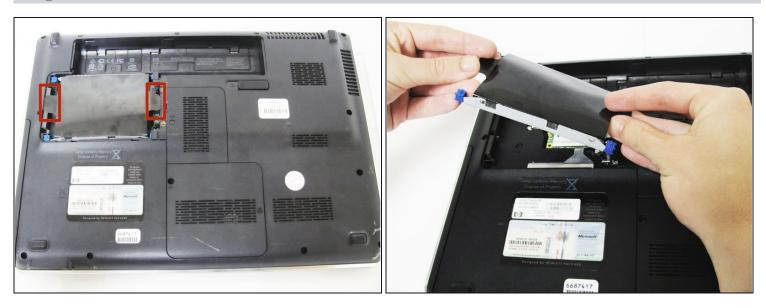
• Pull up on the two plastic flaps on the hard drive enclosure to remove it.
