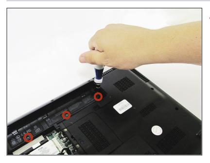
Begin by unscrewing the three 3mm Phillips head screws inside the battery bay with the Phillips #00 screwdriver.
