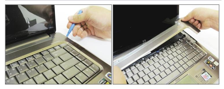
• Flip the laptop, and use the plastic opening tool on the side seam to remove the top cover.
