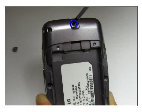
Then, take the pointed end of a spudger and pry out the rubber stopper to reveal the last screw at the top indicated with the blue circle.
