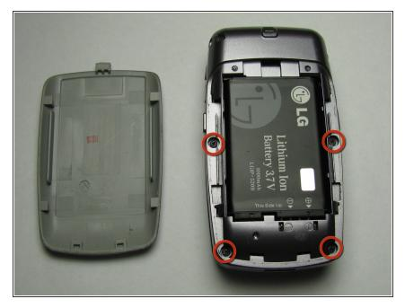
Take the Philips screwdriver and unscrew the four visible screws on the backside of the phone indicated by the four red circles.
