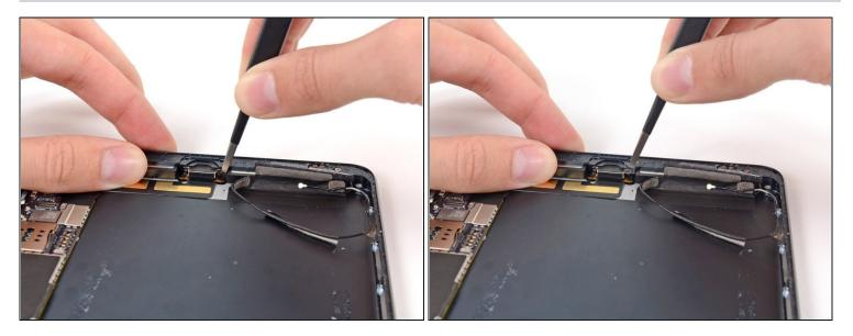
• Remove the plastic covering from the left side of the Lightning connector housing.
