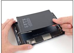
• Lift and remove the battery from the iPad.
