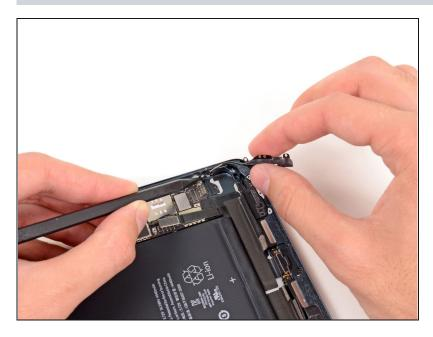
Use the tip of a spudger to pry the small metal retaining clip off the antenna cable, then de-route the cable from the clip.
