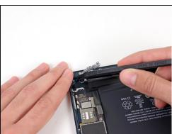
Use the flat end of a spudger to loosen the foam adhesive holding the antenna to the right speaker.
