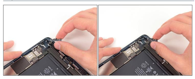
Gently de-route the antenna cable from the bottom right corner of the rear case.
