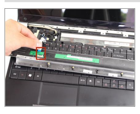
Disconnect the dark colored locking tab by pulling at a 90 degree angle, and then slightly pull away the ribbon from the locking tab.
