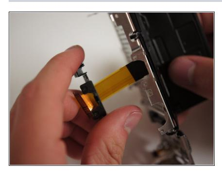
Turn the assembly around and slide the plastic cover off of the ribbon cable.
