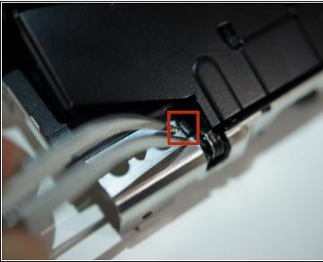
Use the tweezers to push the tab near the bottom left corner of the panel to release a plastic cover from the back of the panel.
