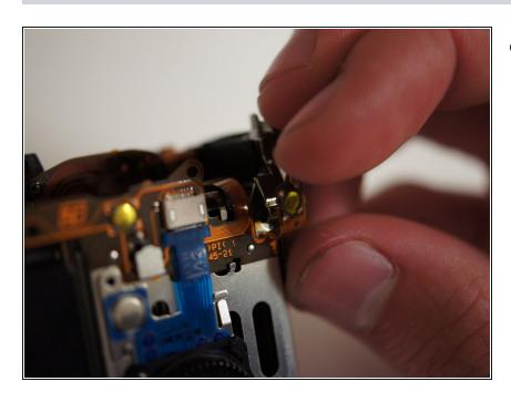
Before pulling off the assembly, fold the rightmost tab of the flexible circuit board away from the metal bracket.
