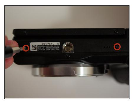
Start by removing the two 5/32" #00 screws on the bottom of the camera using the Phillips #00 screwdriver.
