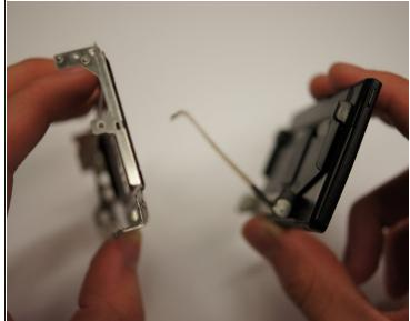
• Remove the screen from the metal panel.
