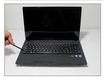
Remove three screws on bottom of case. They have a little keyboard image next to them. If you don't do this first, the keyboard will not come off. Place the plastic spudger right under the edge of the keyboard and lift up the keyboard.
