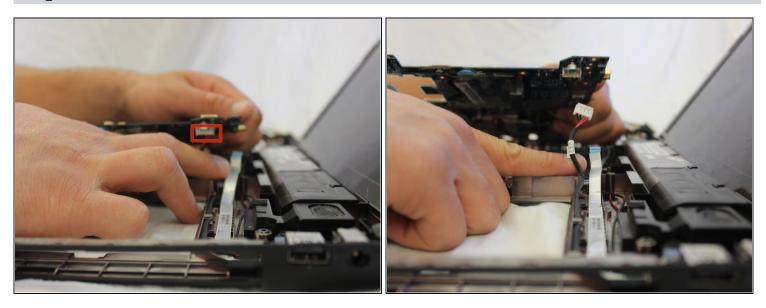
• Remove final plug connecting motherboard to base of laptop.
