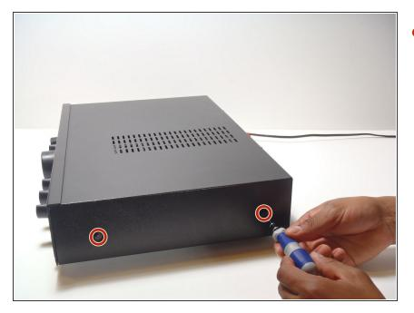
Remove 2 screws from each side of the amplifier.
