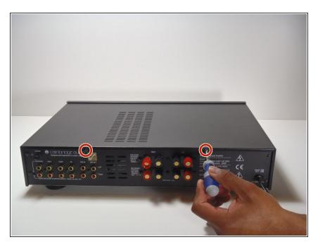
Remove 2 screws on rear of device.
