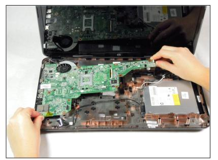
Lift the right side of the motherboard up at roughly a 45 degree angle and pull to the right to remove it.
