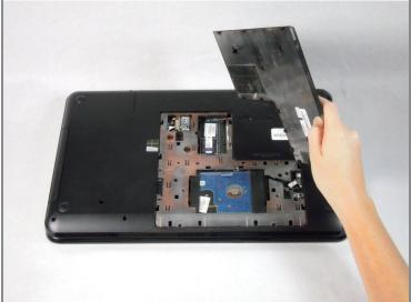
Slide the back panel down and pull it up.
