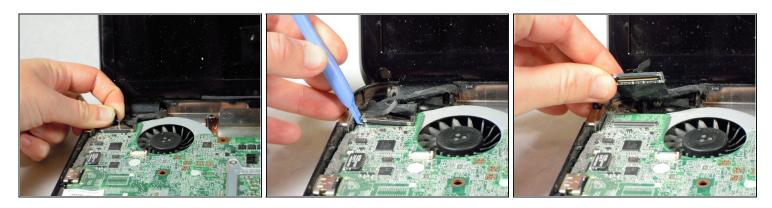
• Lift, with your fingers or a plastic opening tool, the large black monitor cable at the top of the left hand corner of the motherboard.
