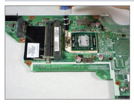
Using a flat head screwdriver or spudger, turn the black plastic tab screw away from the CPU.
