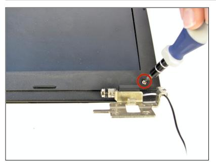
Use the Phillips #0 screwdriver to remove the two 4.8 mm Phillips #0 screws.
