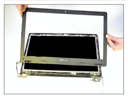
Once pried away from the back bezel, the front bezel will easily lift away from the LCD.
