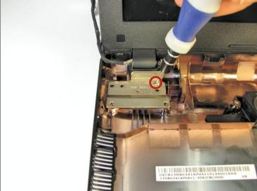
• Use the Phillips #0 screwdriver to unscrew the two 4.8 mm Phillips #0 screws on the right hinge, and the one 4.8 mm Phillips #0 screw on the left hinge.
