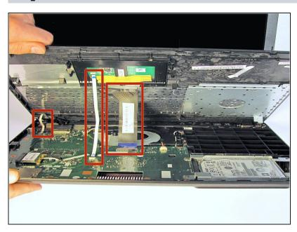
Locate the three ribbons connecting the keyboard plate cover to the bottom cover.
