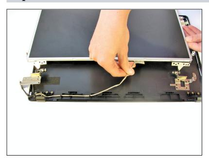
Gently unhook the wire from the back bezel to allow the LCD to be flipped over.
