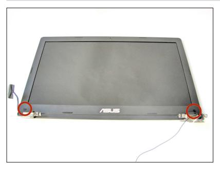
Locate the two stickers that cover up the screws that hold the front bezel in place
