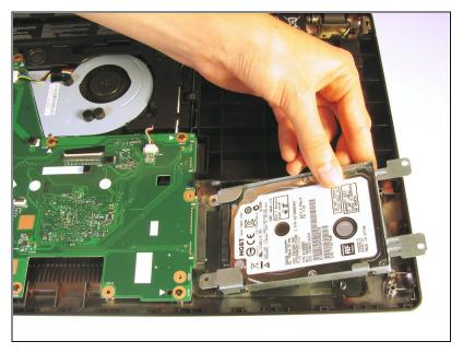
• Once it is free, remove the hard drive from its internal cavity.
