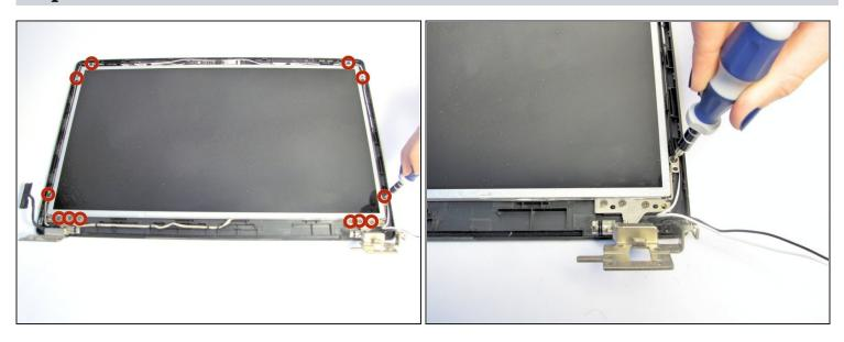
• Use the Philips #0 screwdriver to remove the twelve 3.2 mm Phillips #0 screws that hold the LCD in place.
