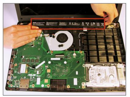
Remove the battery from the laptop by applying pressure on both ends and lifting it out of the case.
