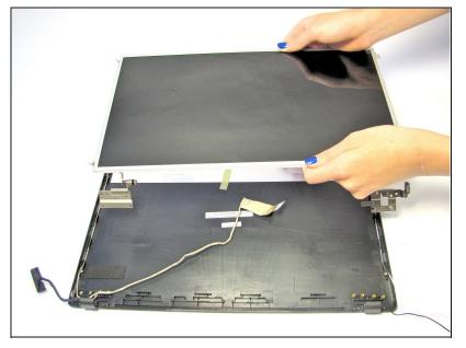
Now that the ribbon has been detached from the back, carefully remove the LCD.
