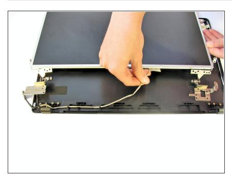
Gently unhook the wire from the back bezel to allow the LCD to be flipped over.
