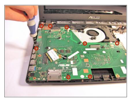
With the Phillips #0 Screwdriver, remove the nine 5.5 mm Phillips #0 screws which hold the motherboard in place.
