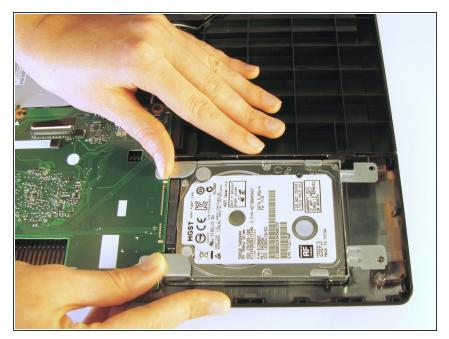
Once the screws have been removed, place your fingers on the left corners and push the hard drive towards the right edge of the laptop (relative to the picture).
