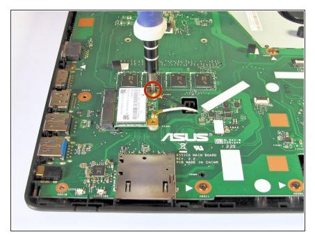
Use the Phillips #0 Screwdriver to unscrew the 3.2 mm Phillips #0 screw which attaches the WiFi card to the motherboard.
