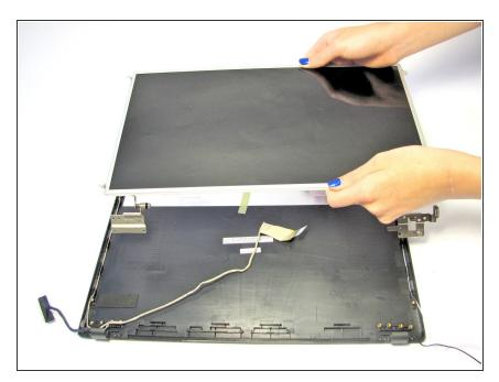
Now that the ribbon has been detached from the back, carefully remove the LCD.
