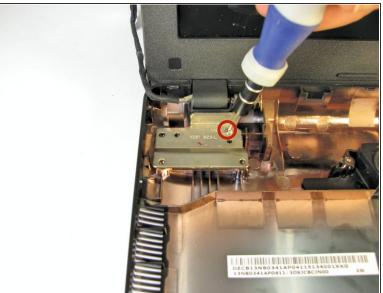
• Use the Phillips #0 screwdriver to unscrew the two 4.8 mm Phillips #0 screws on the right hinge, and the one 4.8 mm Phillips #0 screw on the left hinge.
