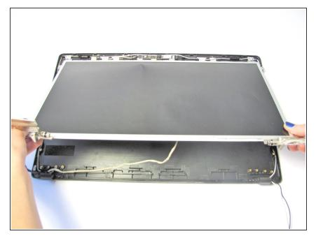
Once the screws are removed, lift up the LCD to expose the wire connecting the back bezel to the LCD.
