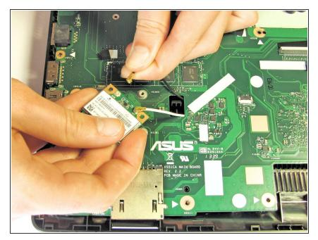
Remove each of the two small antenna connections by disconnecting one wire at a time.
