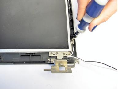
Use the Philips #0 screwdriver to remove the twelve 3.2 mm Phillips #0 screws that hold the LCD in place.
