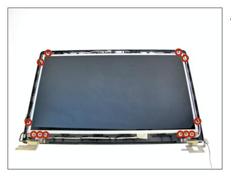
Locate the twelve 3.2 mm Phillips #0 screws that hold the LCD in place.
