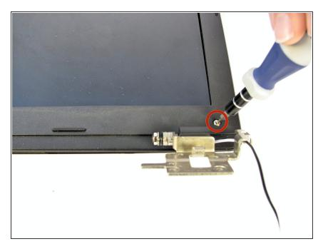
Use the Phillips #0 screwdriver to remove the two 4.8 mm Phillips #0 screws.
