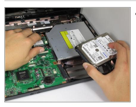
Lift and remove the hard drive from the laptop.
