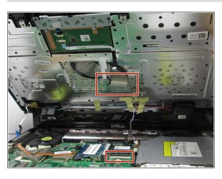
Flip up the small locking flap on the keyboard cable ZIF socket and disconnect the keyboard ribbon cable.
