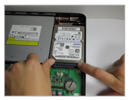
Position your fingers on two sides of the hard drive in the bottom right corner of the computer.
