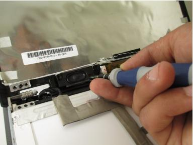
Remove the 2 pairs of 1.5 mm Phillips #1 screws on the speakers.
