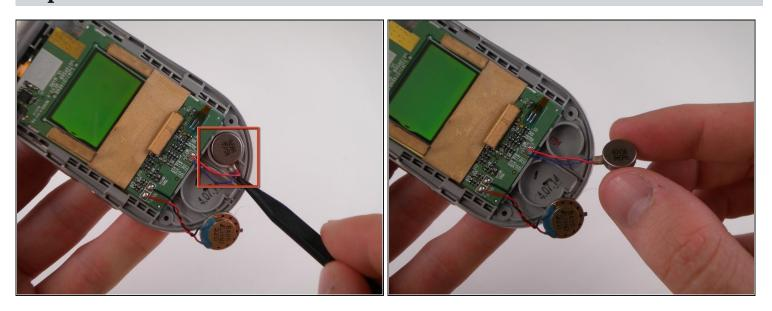
• Remove vibrator using the Spudger.
