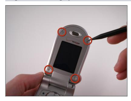
Remove 4 rubber grommets using the Spudger.
