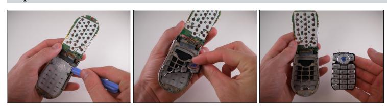
Use an iPod Opening Tool to lift up on the keypad and pull it out.
