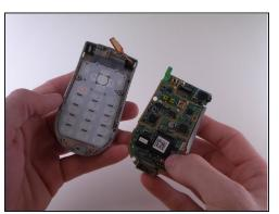
• Carefully detach the ribbon cable and remove the motherboard.
