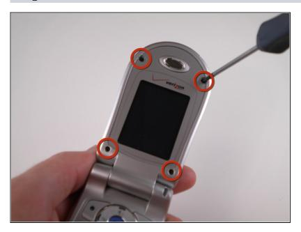
• Remove 4 screws using the Phillips #00 Screwdriver.
