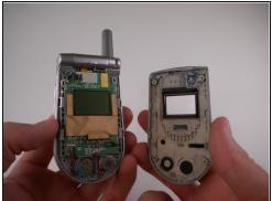
• Carefully pry off outer cover using iPod Opening Tool.
