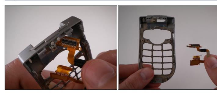
• Remove cable from bottom section.
