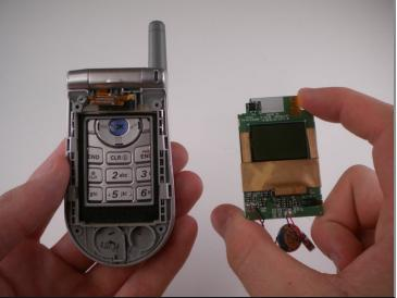
• Pry off ribbon cable using iPod Opening Tool.
