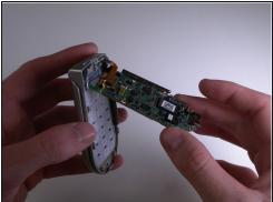
• Carefully pry and lift up on the logic board using an iPod Opening Tool.
