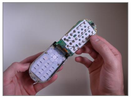
• Carefully flip the logic board up and out of the way.
