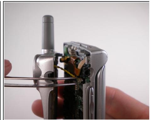
⚠ When removing back cover, be careful not to break the speaker wires.
