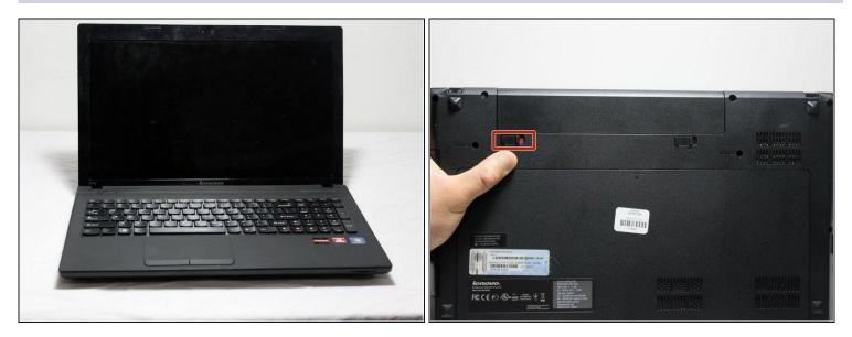
• To unlock the battery, flip the laptop over so that the bottom is facing upward. Then unlock the left clip by pushing the clip to the left.
