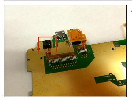
The camera is located on the backside of the system board.
