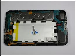
Working slowly and carefully, move around the entirety of the face of the device. Small plastic clips should release, if not, apply gentle outwards pressure until you hear the clips popping off.
