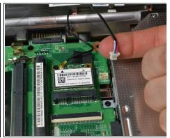
• Disconnect the white block of wires which is the right-most wire connecting the covering to the laptop.
