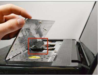
After the top edge of the keyboard is loose, pull up on the keyboard gently.
