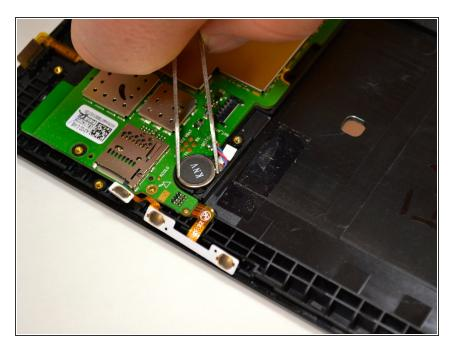
Remove the circular motor unit by gently pulling up on it and prying it up using tweezers.
