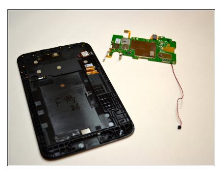
The system board is now completely free from the device. Carefully lift the system board up off of the device and place on a padded surface. To reassemble your device, follow these instructions in reverse order.
