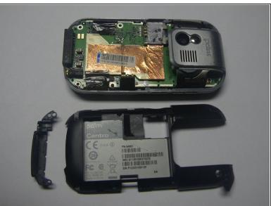
Continue with plastic pry tool all the way around the phone to remove the back housing.
