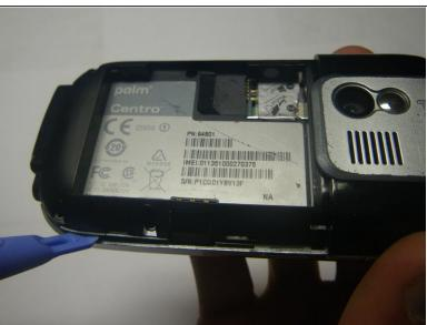
Use a plastic pry tool to separate the bottom of the case to remove the small plastic insert.
