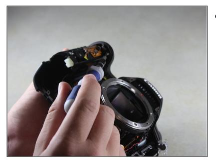
• Remove the 4mm Phillips #00 screw from the inside of the top panel, below the shutter button.
