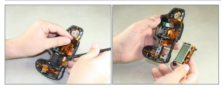
• Carefully slide the flat end of the spudger underneath the screen and lift it out.
