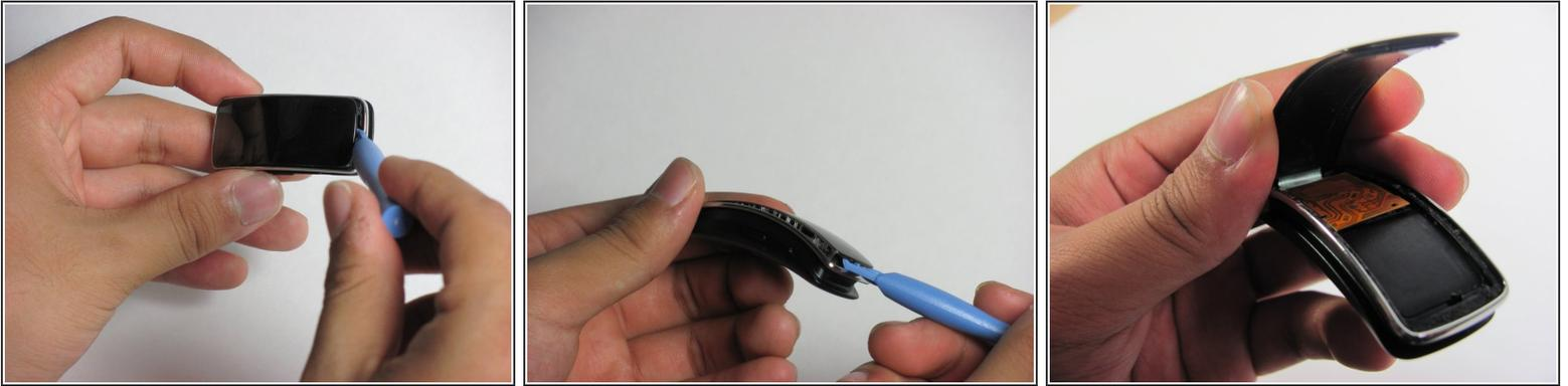
**⚠** The screen is connected to the device by a ribbon cable on the left side with the power button facing you. Do not try to completely separate the screen from the device yet, and be careful.
