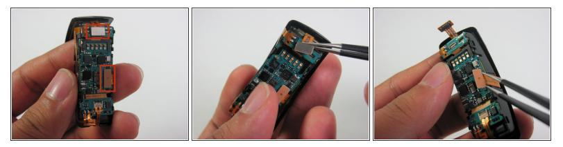
Disconnect the ribbon cables connecting the screen to the motherboard by lifting their metal connectors up off of the board with tweezers.
