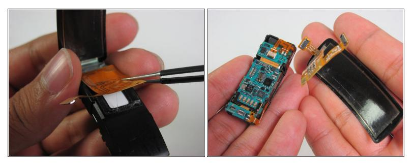
• Gently peel the screen assembly up and away from the device using tweezers.
