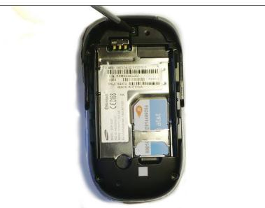
Remove the five screws with a size 00 screwdriver. There are 4 in the corners and one on the top as shown.
