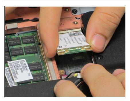
Gently lift the wifi card up to a 45 degree angle from the side with screws.
