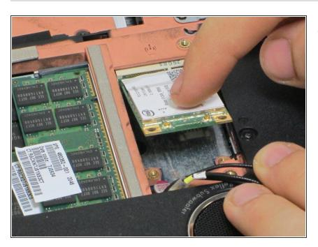
Gently push the wifi card down until the screws can be replaced.
