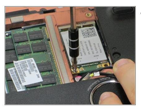
Remove the two Phillips head screws located on the battery compartment side of the wifi card.
