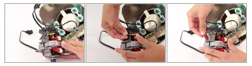
• Now, turn the motor over, and remove the black wire from the motor.
