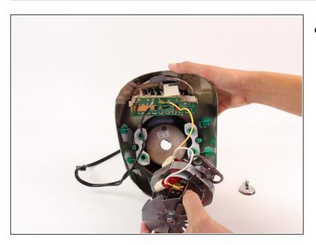
• Carefully remove the motor and fan from the base of the blender.
