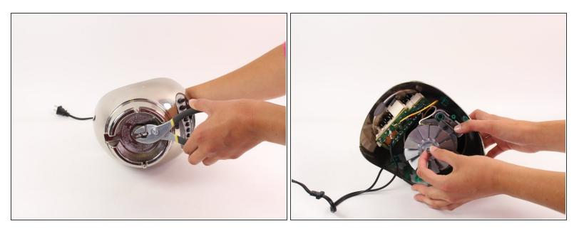
Holding the center of the fan, grip the knob in the center of the top of the blender with a wrench and twist the wrench counterclockwise.
