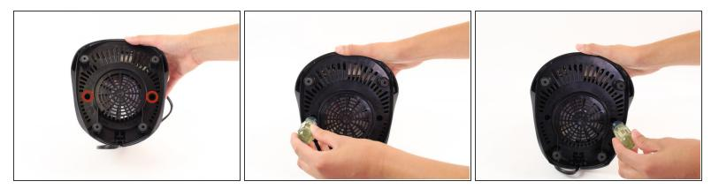
Unscrew the 16mm screws located on the plastic bottom from the blender base using a Phillips #2 screwdriver.
