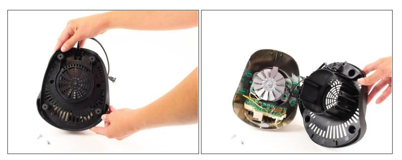
• Remove the plastic bottom from the base of the blender.
