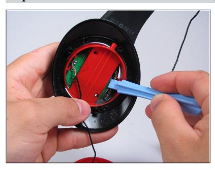
i Sometimes the motherboard will just fall out of its housing. If it doesn't, use a plastic opening tool to gently pry or push out.
