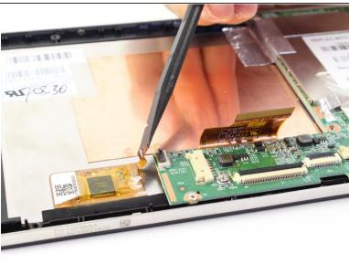
Likewise, disconnect the square radio chip ribbon by lifting up the black panel with a spudger and sliding the gold strip out.
