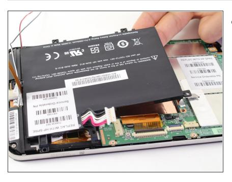
Lift battery out of its place and set aside.
