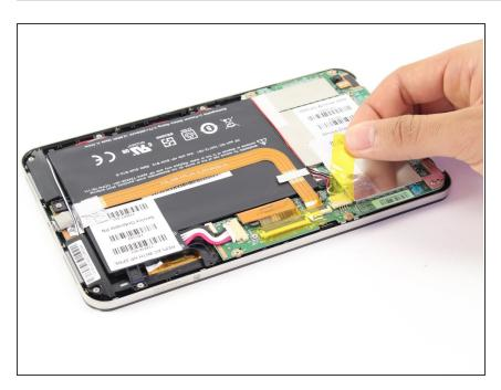
Locate and remove the yellow tape covering the red and white speaker wires.
