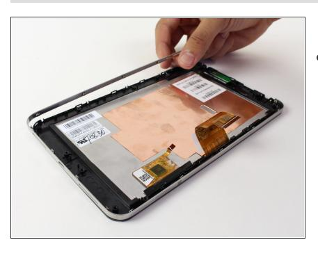
Remove the metal band surrounding the device by lifting it up out of the placement pins. Begin at one end and work your way around.
