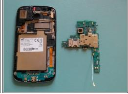
Use a plastic opening tool to remove the motherboard.
