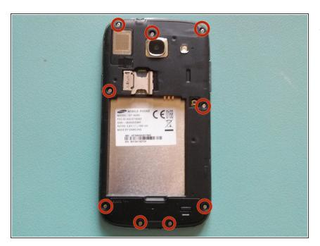
Remove the 9 Phillips #00 screws from the mid-frame.
