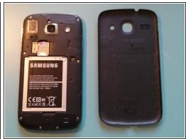
Flip the phone over and use your fingernail or an opening tool to remove the back cover.
