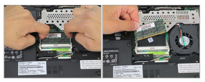
Repeat the process from the previous step to remove the bottom RAM.
