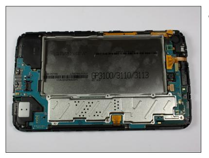
To finish battery replacement, place your new battery where the old battery was in your device, as shown in the picture.
