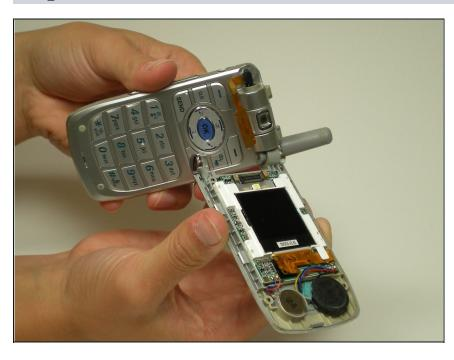
Align new face plate in correct orientation in order to install.
