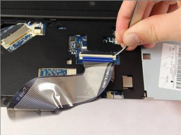
• Using tweezers pull the white tab down on both sides. This will release the blue and black connector.
