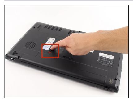
"Unlock" your battery by moving the switch as shown so that an unlocked lock on a red background is shown.
