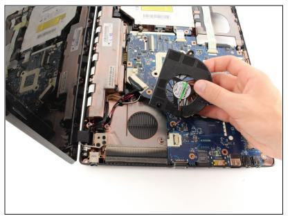
• Carefully lift the fan out of place.
