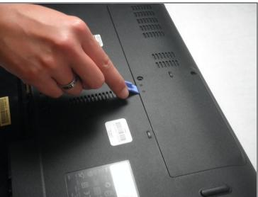
• Once both screws have been removed use a plastic opening tool to lift the panel up. Starting with the indented notch, and moving left and right from there.
