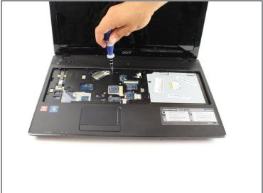
• Flip the Laptop back over, and unscrew the 1/4" diameter head 7/32" length screws indicated in the picture.
