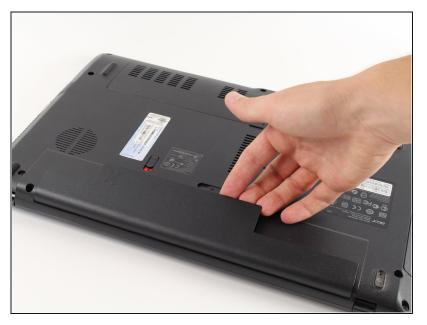
Now remove the battery by lifting it out of the laptop by the side closest to the switches.
