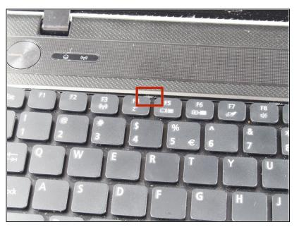
Locate the tabs keeping the keyboard in place.
