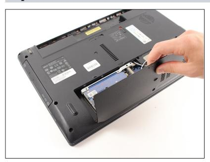
After the panel has been loosened by the plastic opening tool, take your finger, place it in the gap, and remove the panel from the laptop.
