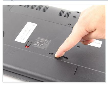
Next move the other switch, while the unlocked symbol is still showing. The battery should pop up, and no longer be flush with the bottom of the laptop.
