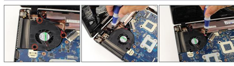
• Once you manage to locate the fan use the screwdriver to unscrew the three screws highlighted.
