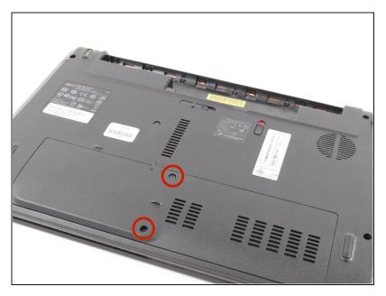
Now, locate the two screws that hold the back cover panel onto the laptop.
