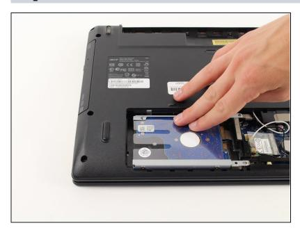
Carefully slide the hard drive in the opposite direction of where the screws are located until it dislocates.
