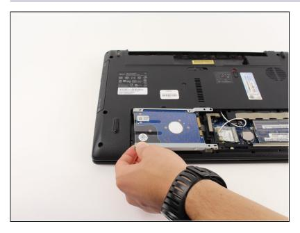
Pull the hard drive out of its compartment.
