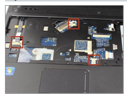
• The indicated spots show where different components are attached to the motherboard (such as the power button and the track pad). You will have to remove these connections the same way you undid the keyboard using the tweezers.
