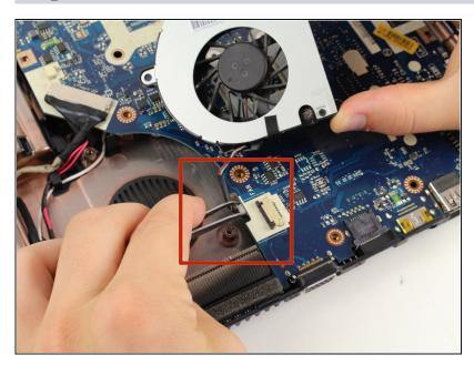
Use tweezers to disconnect the wires connecting the fan to the laptop.
