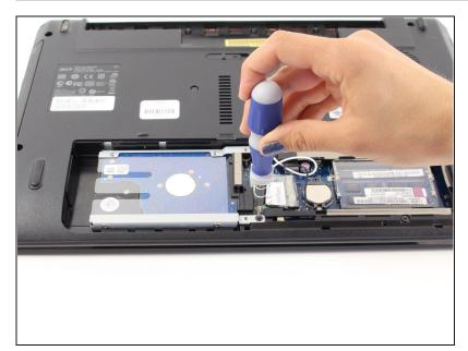
• Remove the two screws using a Phillips #00 screw driver.
