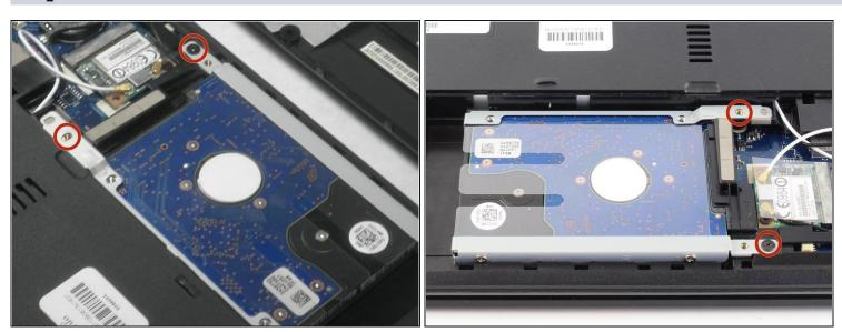
• Locate the two screws that are holding the hard drive in place.
