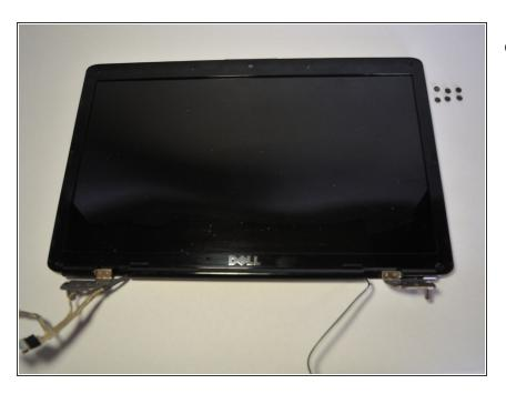
Lift the display assembly off the computer.
