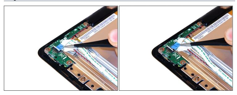
• Pull the connection apparatus from the connection clip on the board using a pair of tweezers.
