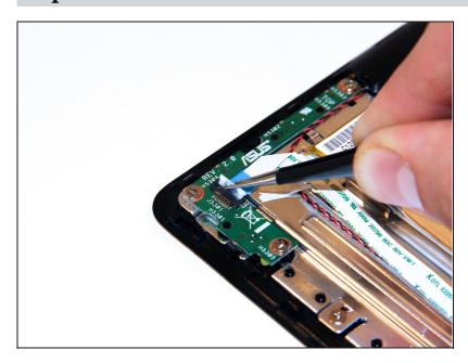
• Unclip the white connection clip using a pair of <u>tweezers</u>.
