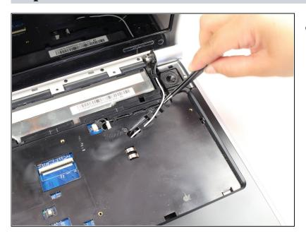
Using the <u>tweezers</u>, pull out the black and white cables located at the right side of the laptop.
