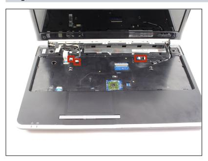
Locate the three LCD connectors.
