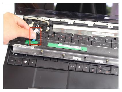
Disconnect the dark colored locking tab by pulling at a 90 degree angle, and then slightly pull away the ribbon from the locking tab.
