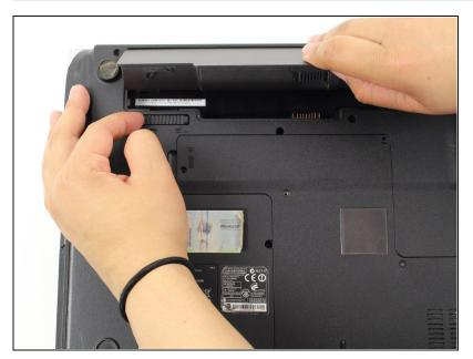
Slide the horizontal latch to the right to pop open the battery pack.
