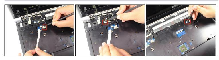
Use the pointy end of the spudger to gently pry each side of the LCD connector until they are detached from their respective ports.
