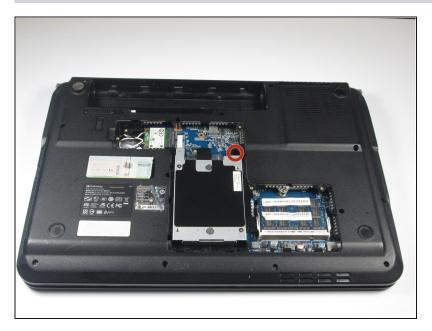
• Remove the 1/4" Phillips #0 screw located at the top right of the hard drive.
