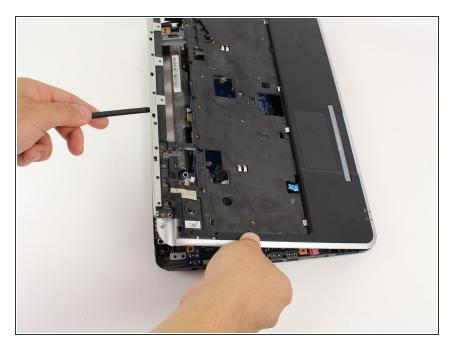
Separate the top cover from the base using the heavy duty spudger. Insert the spudger in between the keyboard base and the base of the laptop with a minimum amount of force to separate them. Follow this procedure around the perimeter until the parts are separated.
