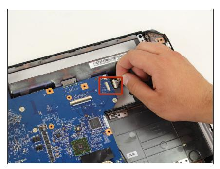
Cautiously disconnect the USB board cable that is situated on the top right corner of the motherboard.
