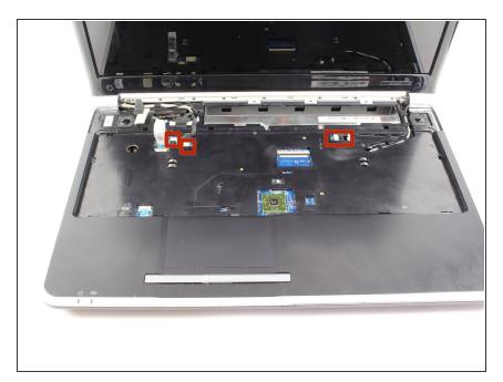
Locate the three LCD connectors.
