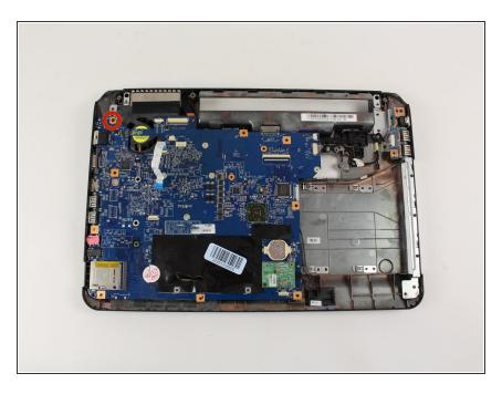
Remove the 3/16" screw securing the motherboard with a Phillips #0 screwdriver.
