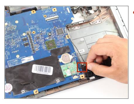
Disconnect the modem cable located at the bottom right of the motherboard.
